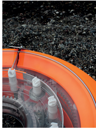
A semi-automatic knitting machine, operated by the current, drifting self-sufficient in the sea.
